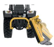
1 HYDRAULIC SHOCK ABSORBER TRILAT flails feature a shock absorbing system on the angle ram which protects the machine in work and allows the flail head to float and follow the contours.
