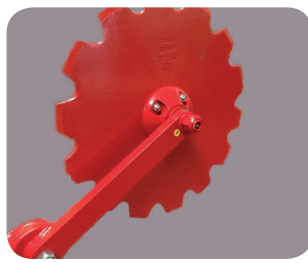
Smooth or scalloped disc coulters. (Pair of smooth discs standard on rear furrow in the UK)
