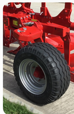
Rear depth and transport combi wheel 340/55 (Standard on 150 & 180 ploughs in the UK)
