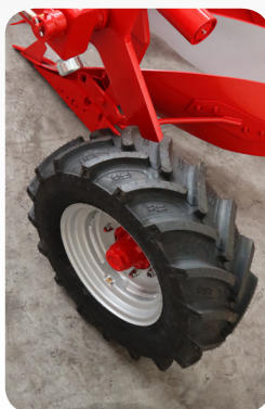
Rear depth control wheel 280/70 (Standard on 130 ploughs in the UK)
