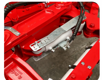
Hydraulic front furrow width adjustment. (Standard on all Xperience ploughs in the UK)
